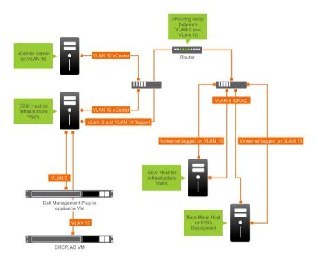
Figure 4. Example VLAN network.
